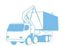
6m Side Loader Clearance Requirements Height – 4.5m (15') Width – 6m (20') Length – 10m (33')
